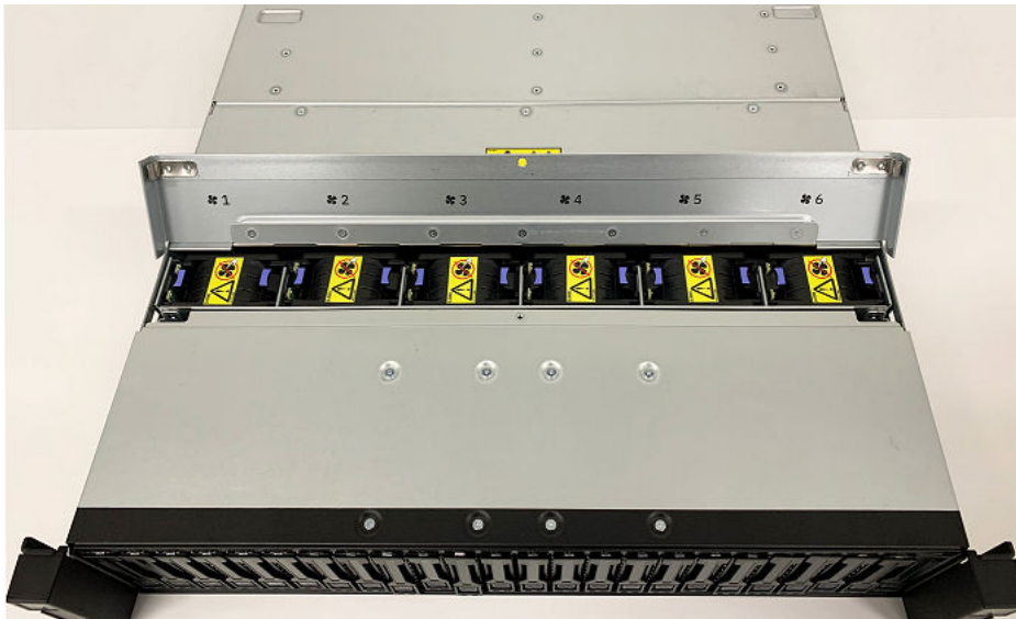
Figure 68. IBM Elastic Storage System 3500 fan LEDs
