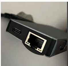
Figure 123. Adapter slot to access server via Ethernet
