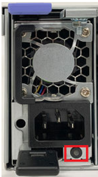
Figure 69. IBM Elastic Storage System 3500 power module status LED
