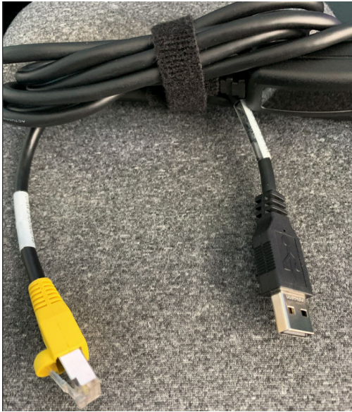
Figure 119. POWER9 EMS (serial to USB)
