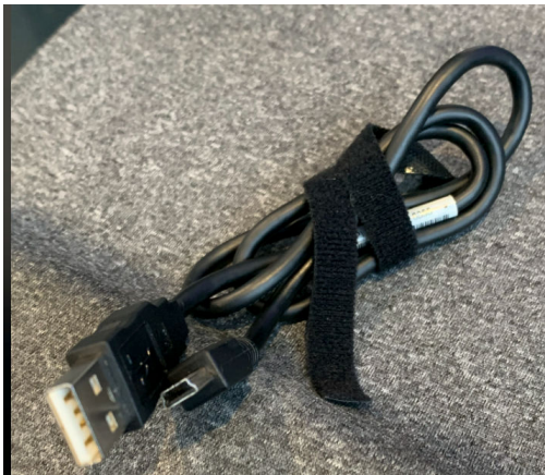
Figure 118. Serial (USB mini-B) to USB cable
