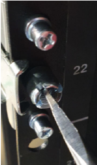
Figure 43. Securing the front of the rails
